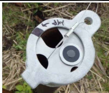
An observation well equipped with a data logger.
