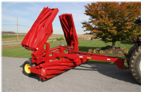
Above picture is an example of a roller crimper that is similar to the one used by Stoney Brook Farms to terminate winter cereal rye cover crop.
